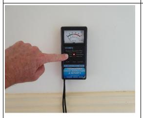
There was no moisture or water leaks located behind the shower when tested with a moisture metre. There was no signs of swelling to the moldings on the outside of the shower at the time of the inspection.
